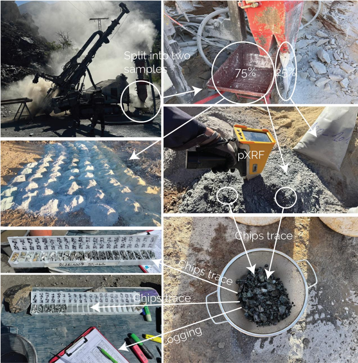
Figure 42. RC Drilling Sample Processing and Logging.
