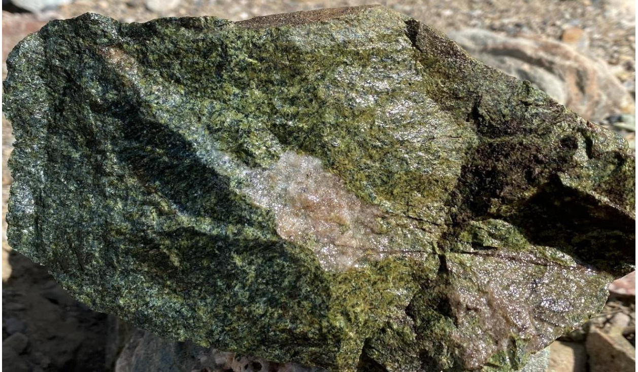
Figure 26. Calc-silicate altered float, likely originating from a subvolcanic formation, accompanied by chlorite, epidote, magnetite, and quartz.
