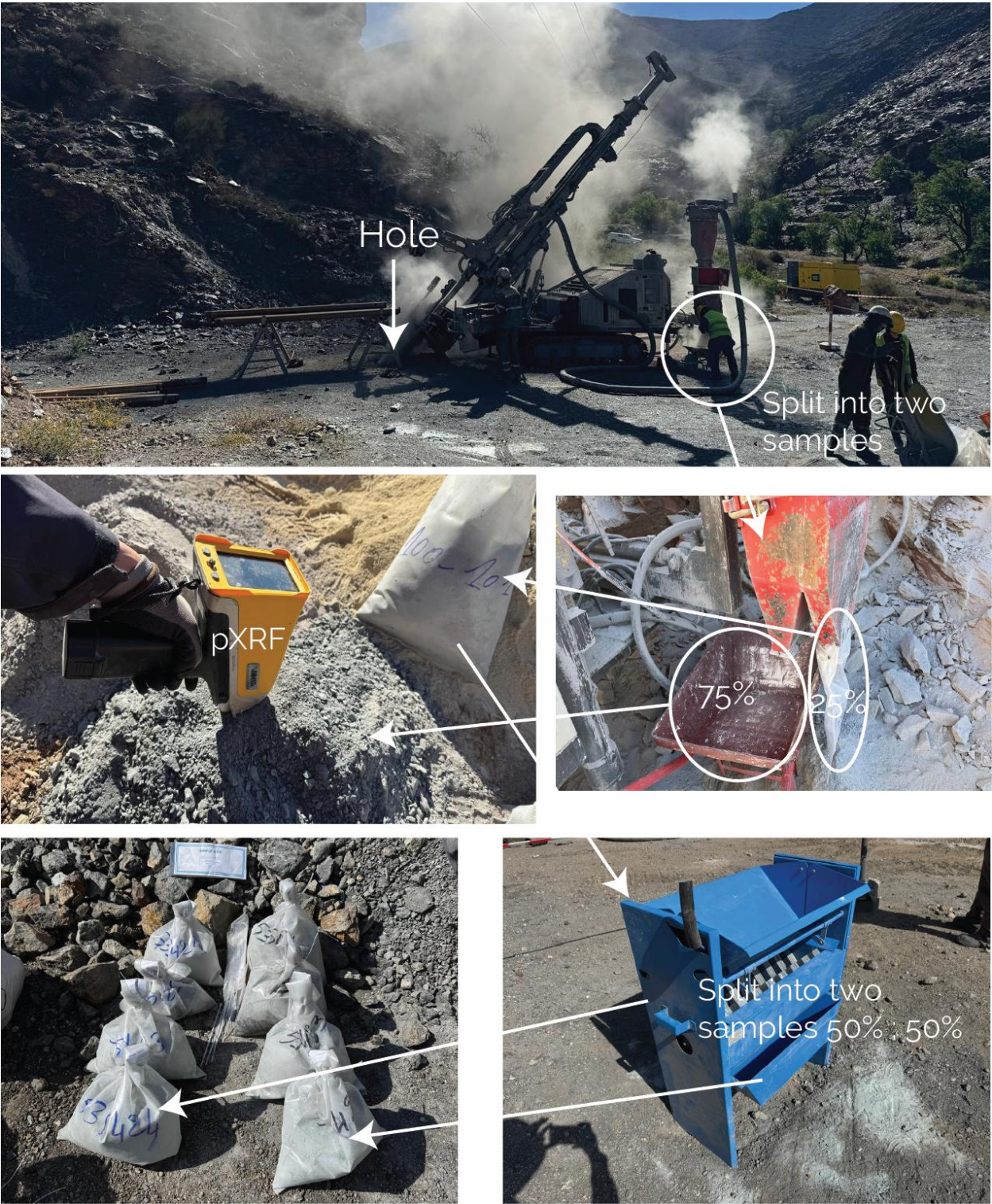
Figure 41. Reverse Circulation (RC) Drilling and Sampling.
