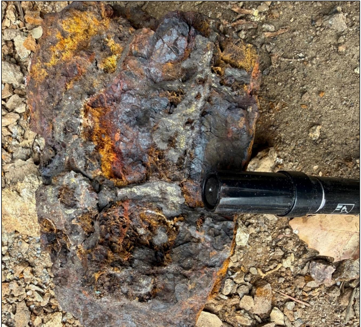
Figure 87: Chalcopyrite-pyrite massive in gossan structure from underground.
