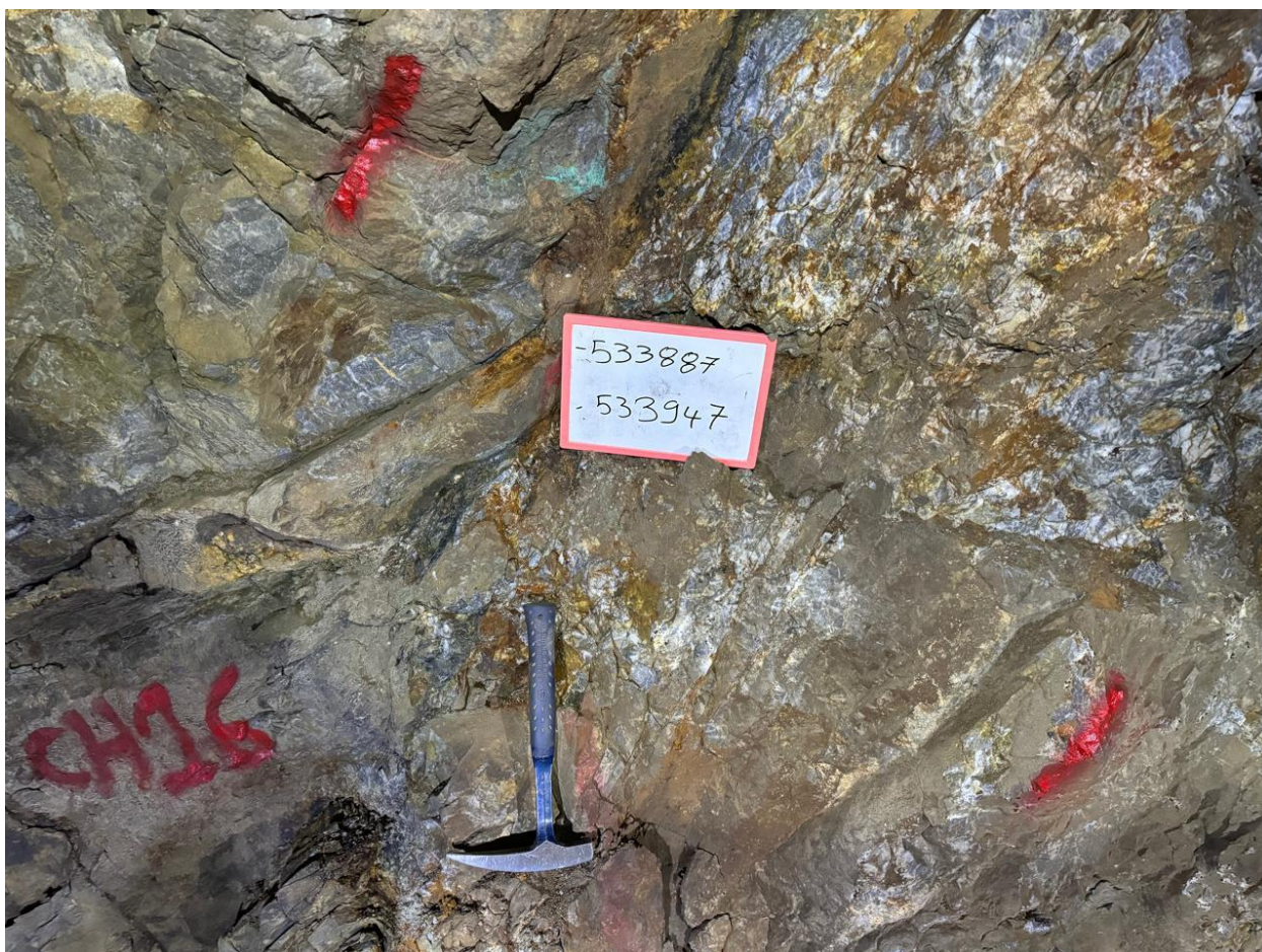
Figure 59. Underground channel sampling.
