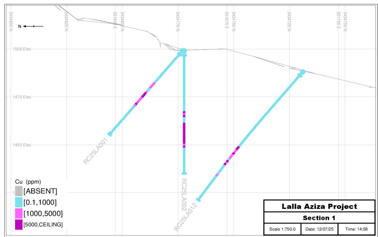
Figure 46. Section 1, Copper (Cu) Assay Distribution in RC Drill Holes, Lalla Aziza Project.
