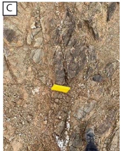
Figure 31. A) Siliceous mineralized vein located within the fault contact between the Lower Dolomite and a low angle shear zone. The vein consists of quartz – malachite – calcite, B) & C) Milky quartz veins along with malachite directly below the main mineralized shear zone hosted ore shoots. The geometry of the veining follows parallel to sub parallel the S0/S1 of the chlorite schists and their general trend varies from N330 to N30.
